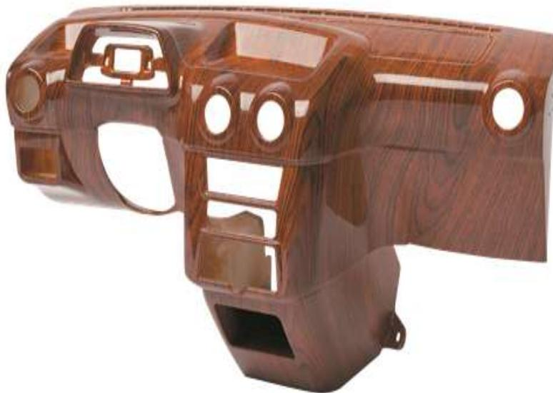
This full-size automotive dashboard was printed in a single piece on an Objet500 Connex 3D printer from Stratasys, then painted with a process known as water-transfer printing. Photo courtesy of Stratasys.
