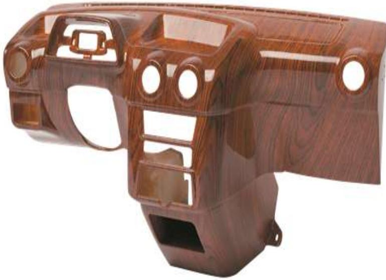
This full-size automotive dashboard was printed in a single piece on an Objet500 Connex 3D printer from Stratasys, then painted with a process known as water-transfer printing. Photo courtesy of Stratasys.
